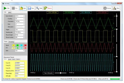
The Fourier transformed spectrum of each signal channel can be displayed after checking the corresponding software control.
