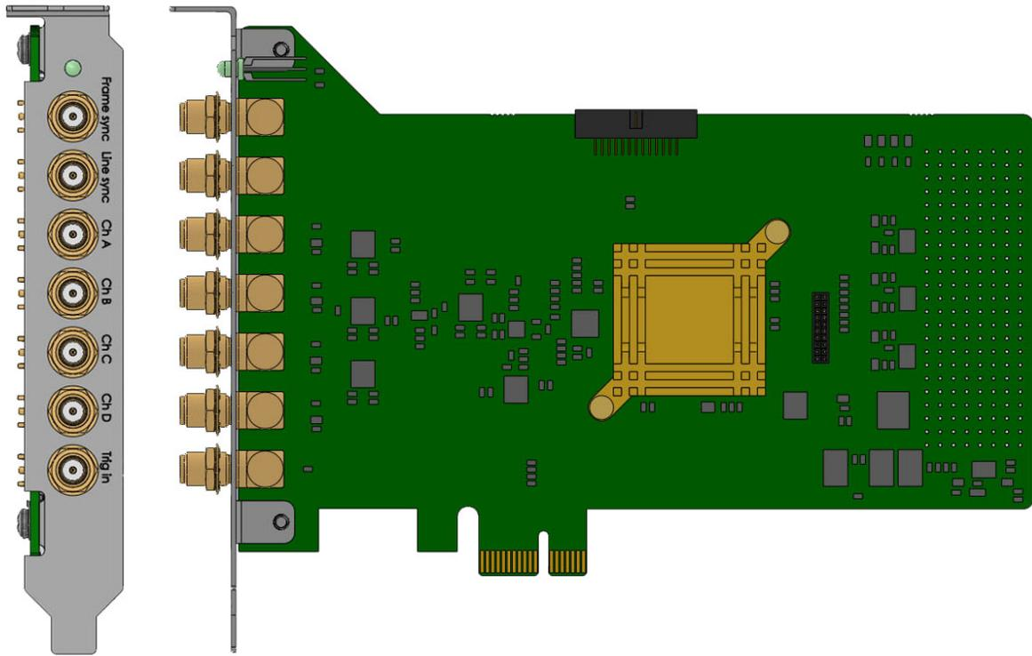
*Product left and front views. There are total 7 SMA connectors on the PCI mounting bracket, and from top to bottom are: (1) Frame sync output, (2) Line sync output, (3) Channel A input, (4) Channel B input, (5) Channel C input, (6) Channel D input, (7) Trig input.*
