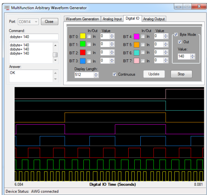
AWG control software user interface: digital output mode. All digital IO bits are configured as one byte to output simultaneously.
